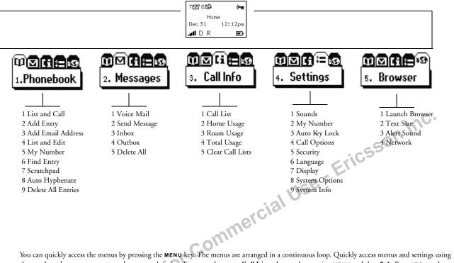
You can quickly access the menus by pressing the **MENU** key. The menus are arranged in a continuous loop. Quickly access menus and settings using the numbers that appear next to each menu and setting. For example, access **Call List** submenu by pressing **MENU** and then **3 1**. Press **YES** to select a menu, submenu, or setting. Press **NO** to exit the menu or submenu.
